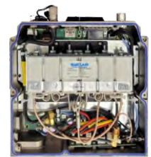
MR3332S-3 Internal Duplexer, 5 MHz separation
